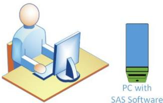
In this diagram, SAS programs execute on the PC, which means usually that the data, the programs, the execution, and the destination for the output are on the same system. The user may be limited by the number of CPU, memory, disk space, or licensed SAS products installed on the system. The user will not, however, experience any network latency between SAS processes and the disk storage.
